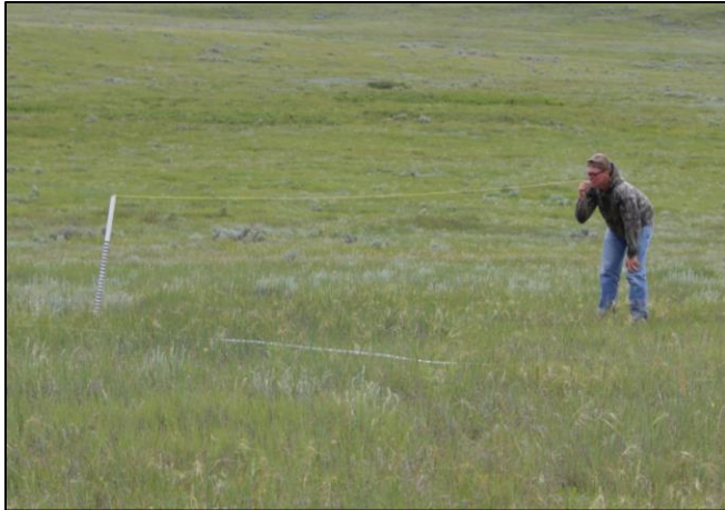
Measuring visual obstruction using a Robel pole
